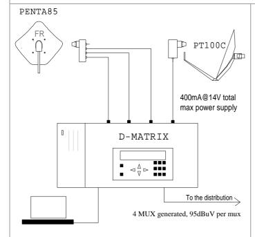
The new D-MATRIX-4S EVO headend can tune up to four different SAT trasponders, decrypt the programs (through CAMs & Smart-Cards – **NOT INCLUDED**) and generate four separate full-band RF Digital Multiplex (DVB-T or DVB-C), 95dB $\mu$ V each.
